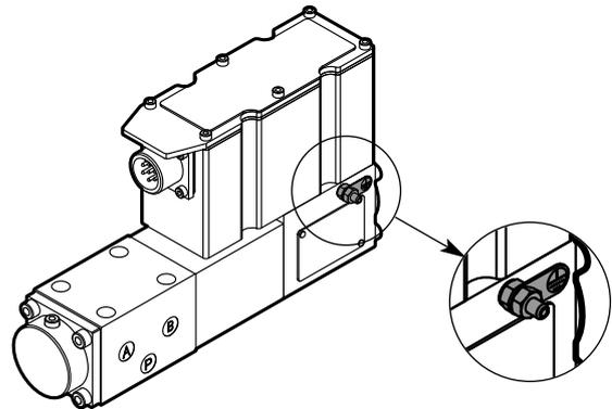
The grounding point must always be wired with the general earthing system by means of a suitable conductive line.
