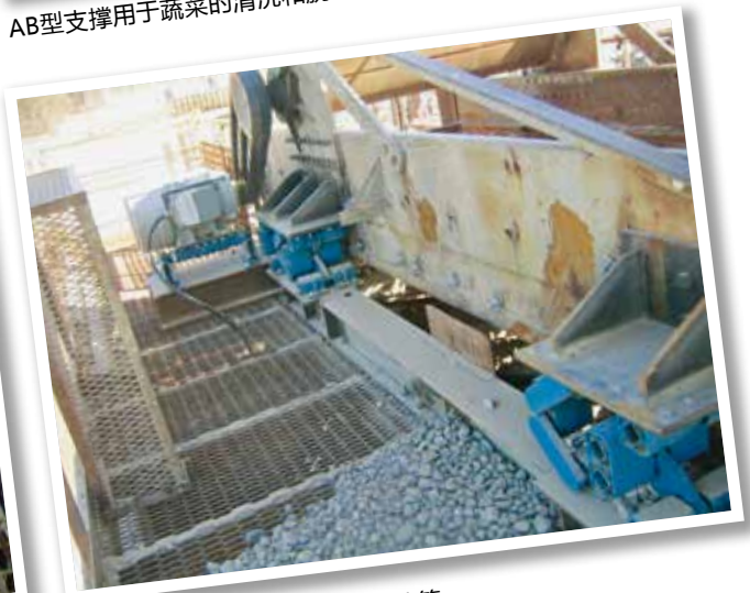
AB TWIN型支撑用于石料圆振动筛
