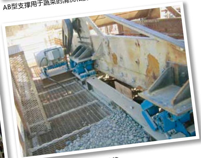
AB TWIN型支撑用于石料圆振动筛
